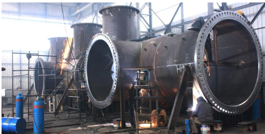
Photo 3. Fabrication of Intake Header (February 2011)
