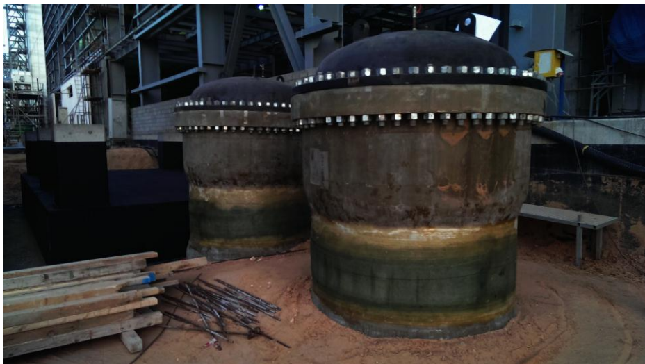
Photo 12. Hydrostatic Site Test of Unit 4 Cooling Water Return Line between Turbine and Surge Chamber with DN1800 Test Covers on Turbine Side (January 2014)
