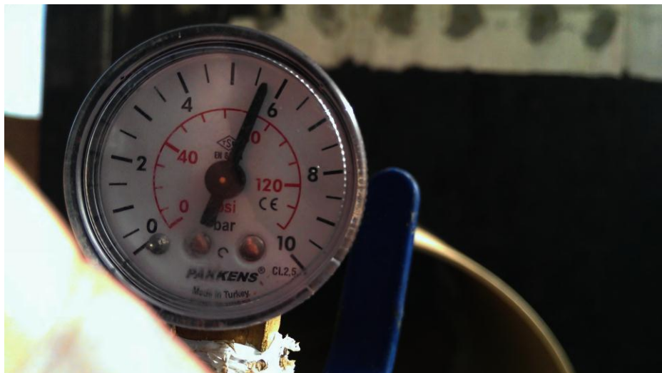
Photo 13. Monitoring of 5.8 barg Site Test Pressure During Hydrostatic Site Test of Unit 4 Cooling Water Return Line between Turbine and Surge Chamber (January 2014)
