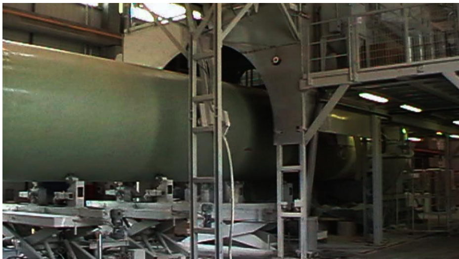
Photo 6. Fabrication of 2500 mm Diameter GRP Pipes (December 2009)
